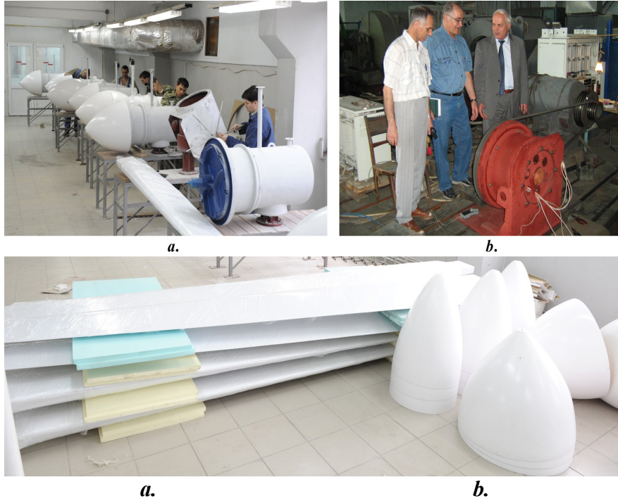
Fig. 4.46. Assembling stage of the component of the wind turbine.
