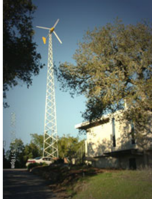
Fig. 4.37. Bergey Excel-S, 10 kW turbine [38].
