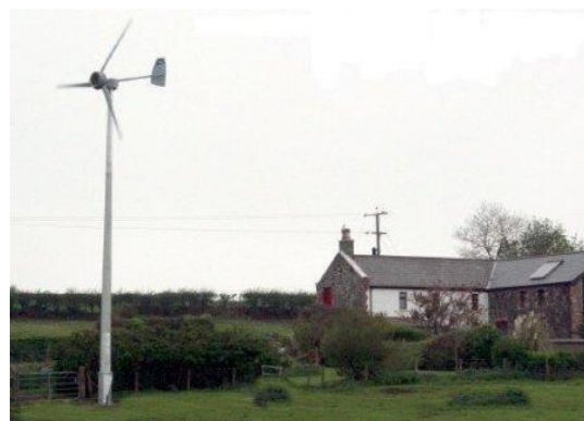
Fig. 4.38. Iskra AT5-1 wind turbine installed near the Redland school, UK [39]
